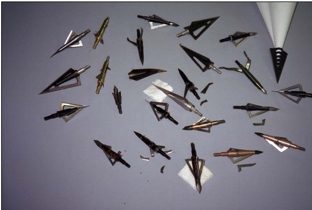
Some of the broadheads damaged during 2004 testing.
