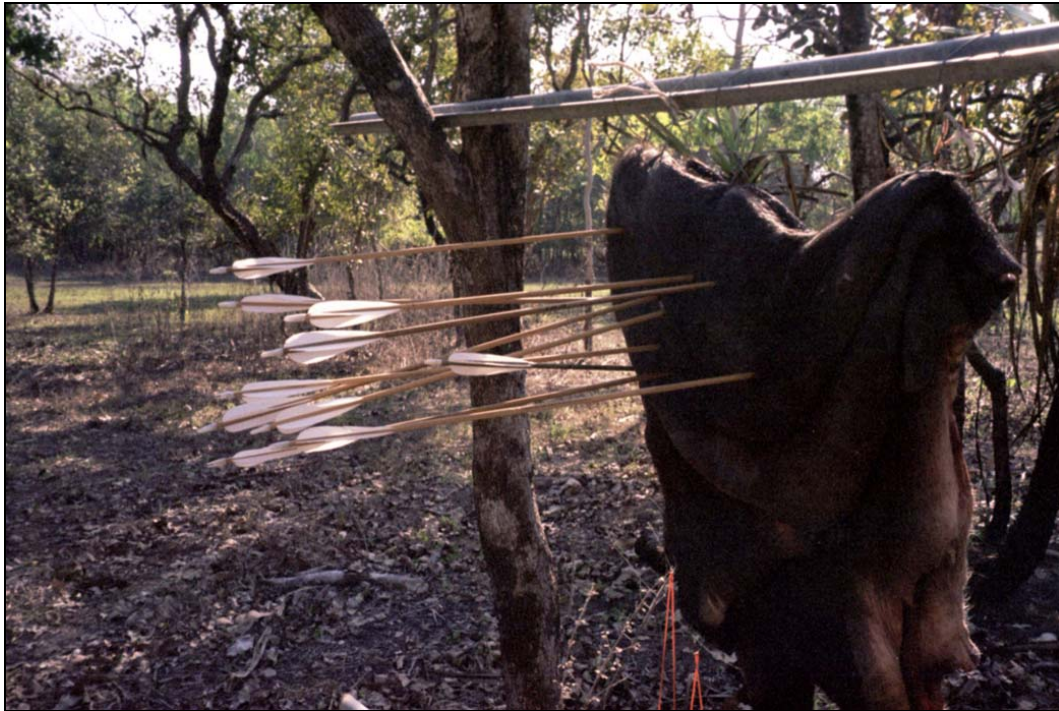
Test shots on buffalo skin. Note penetration of small diameter, double shaft arrow.
