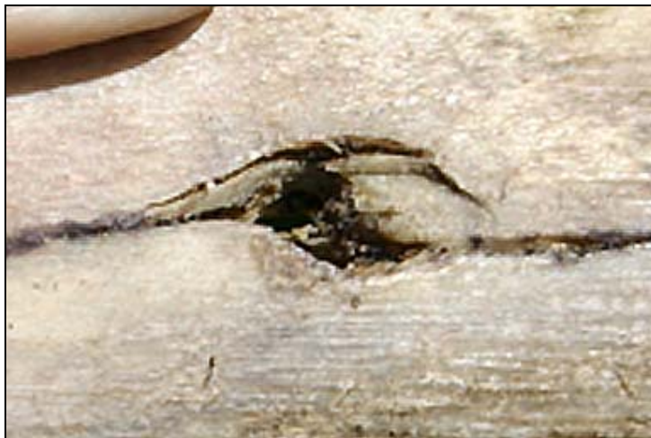
Single bevel induced rotation is clearly visible.
