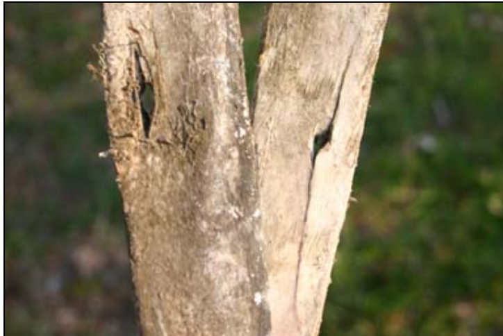
Entrance side; double bevel (Left) and single bevel (Right). Five-inch split (R) was caused by 11/16" wide Grizzly Extreme.
