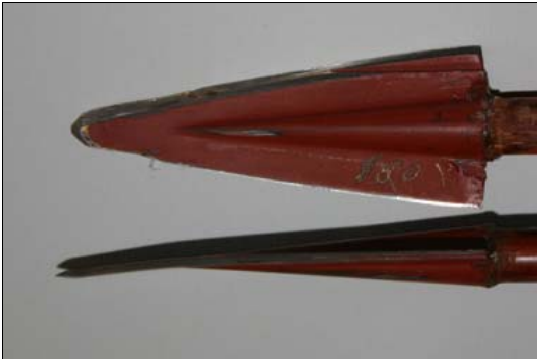
The two bent 160 grain Grizzly broadheads
