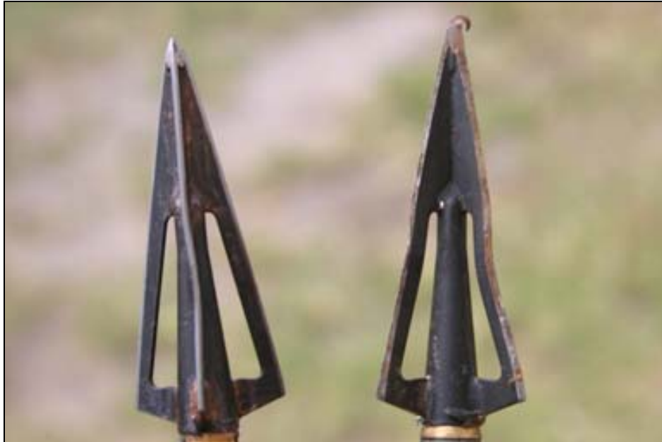
These Wensel Woodsman broadheads were damaged on right-angle rib impact, halting their penetration. Note differing tip design; factory tip (R) curled on every shot while modified tip (L) remained undamaged on all shots.
