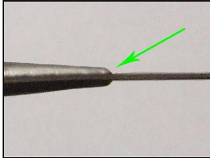
Abrupt ferrule termination often halts penetration in bone. Ferrule taper should fade smoothly into the blade. Irregular surface along the broadhead/arrow profile, whether 'bump, lump, ridge or hole', increases resistance during penetration.
