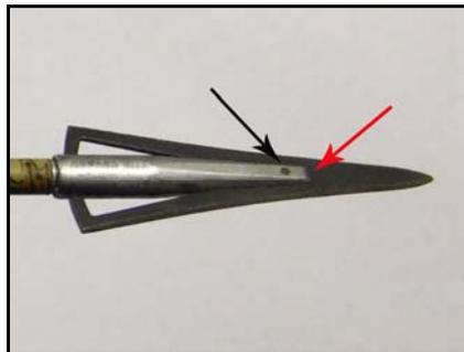
Broadhead strength is an important design feature. Even with excellent blade MA, the Howard Hill Broadhead tends to fracture the ferrule where the retaining rivet (black arrow) passes through. This is more common on angular bone impacts, and there's little doubt that the abrupt ferrule fade-in (red arrow) is a contributing factor to this tendency.
