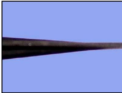
Smooth ferrule fade-in lowers peak resistance force during penetration and increases the MA of the ferrule's wedge-effect.
